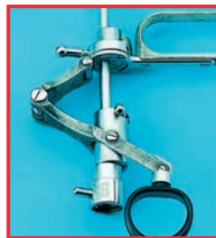
Damage to aluminium components only. Cause: use of highly alkaline detergent
