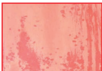
Optical changes to colour anodised aluminium occurs even in mildly alkaline solutions
