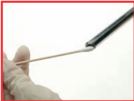
Cleaning the lens of an endoscope
