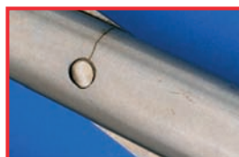
Hairline fracture next to scissor hinge
