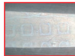
Instrument surface with insert mesh contact pattern
