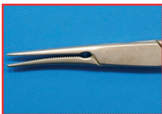
Deformation caused by improper handling
