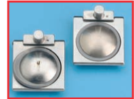
Leaky trocar flap valve due to gasket swelling as a result of oil contact.
