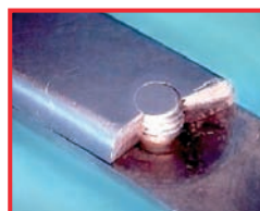
Scissors with breakage around hinge
