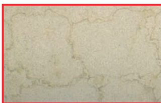
Marbling caused by impurities in steam condensate
