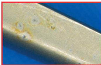
Pitting induced by chlorides on instrument
