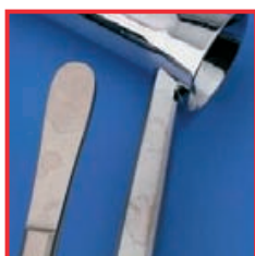
Stains caused by high salt content of rinse water
