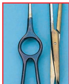
Instruments discoloured by silicic acid
