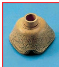
Cracks caused by ageing on breathing mask
