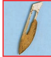
Rust formation on a scalpel blade. Cause: Not stainless steel as this is a disposable product.
