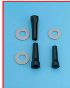
Swollen gaskets as a result of non-targeted instrument oil application.
