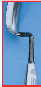
Surgical hook with shaft made of hardened Cr-steel showing black discoloration and handle that has remained bright and blade made of non-hardened CrNi steel
