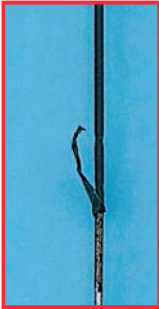
Damaged insulation on HF instrument
