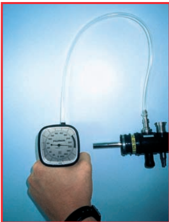
Manual leakage test on flexible endoscope
