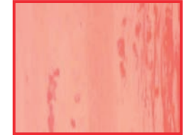
Aluminium surface damage due to use of highly alkaline cleaner
