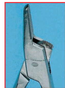
Jaw breakage on suture holder
