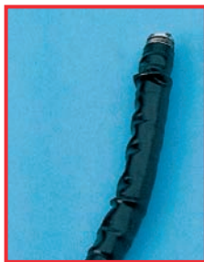
Swelling at distal end of fiberscope
