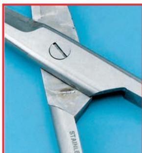
Fretting corrosion due to inadequate lubrication
