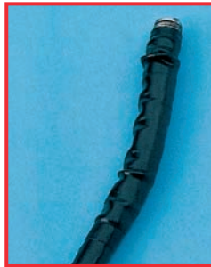
Swelling in a flexible insertion tube due to use of an unsuitable care agent.
