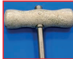
Damage to aluminum handle only. Cause: Use of highly alkaline detergent
