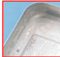
Material attack. Cause: Alkaline cleaner
